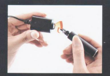
To Charge battery, gently screw battery into the USB charger. Plug USB cable into a USB charger or a computer. Battery should flash to show it is charging. The light on the USB charger is red when charging. Green when fully charged. When using a computer to recharge.
